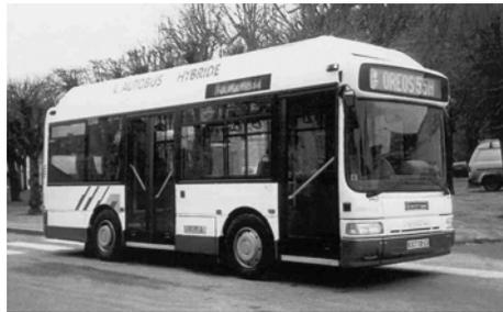
Figure 2 – Hybrid Electric mini-bus OREOS 55 H
