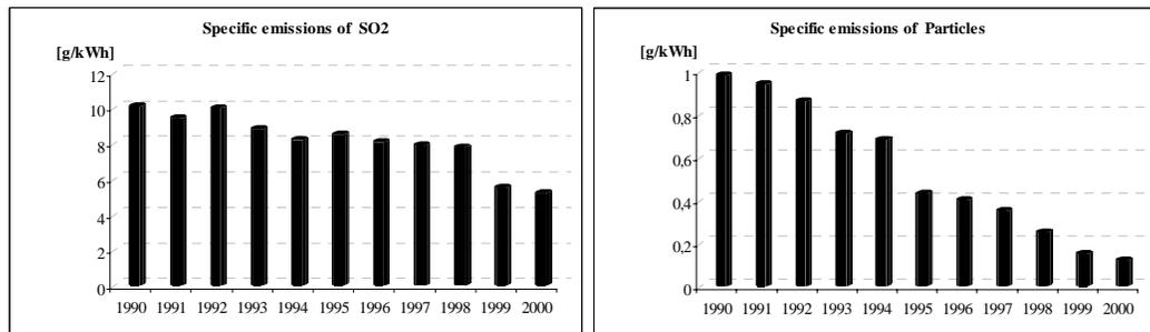
Figure 14 and Figure 15: Evolution of the specific emissions of SO<sub>2</sub> and Particles of the SEN [2]
