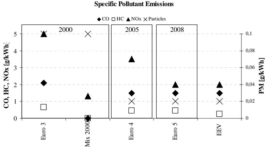
Figure 17: Comparison of specific emissions related to electric and internal combustion mini buses
